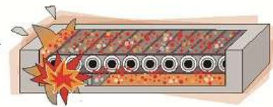
Primary explosion from motor sparking creates dust cloud
