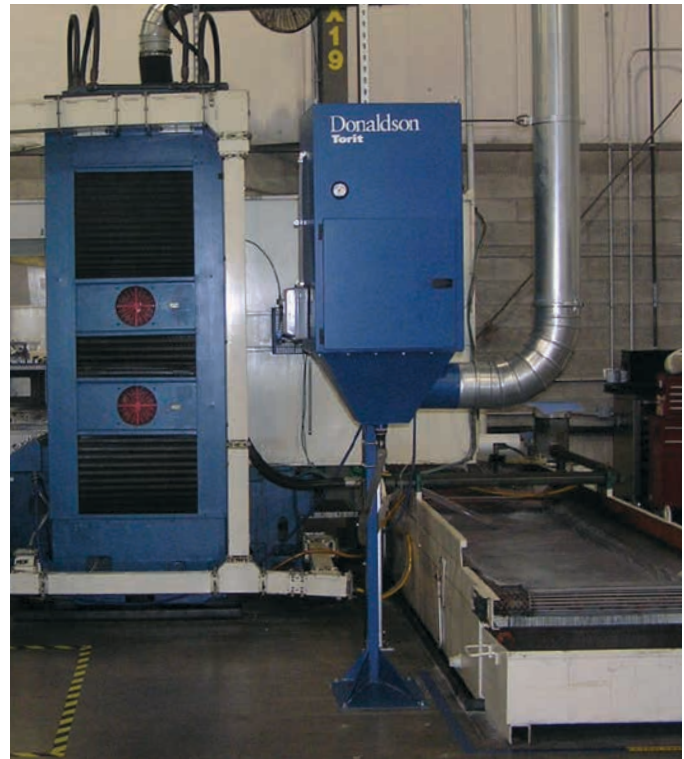
WSO on Water Mist - Horizontal Grinder 850 cfm (1,444 m³/h)
