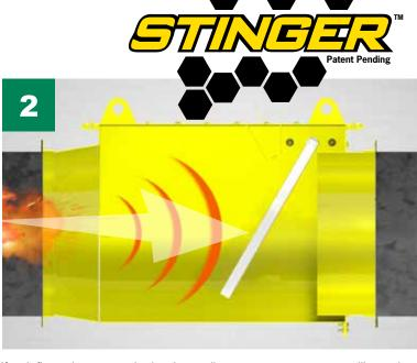
If a deflagration occurs in the dust collector, a pressure wave will travel through the pipe faster than the flame front and close the flap valve.
