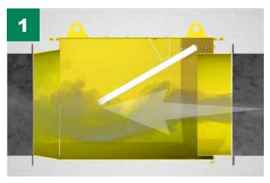
During normal operation, the airflow holds the blade open and a back stop makes sure the blade is in the position that was tested and approved.
