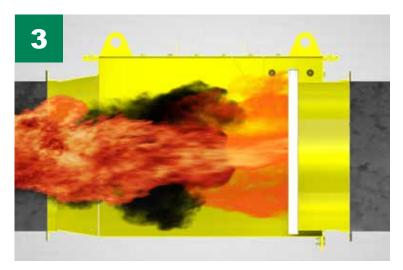
When the valve is fully closed, a latching mechanism keeps it shut. The closed valve prevents the transmission of flame past the valve.
