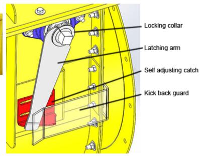
locking mechanism. It provides
