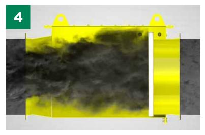
The valve also prevents smoke, dust and burning debris from traveling through the inlet pipe into the factory.
