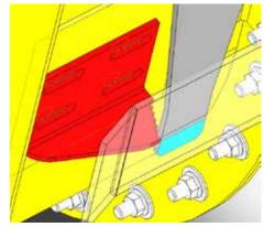
A self-adjusting latching mechanism engages when the valve closes and holds the valve shut during the deflagration. This mechanism will not engage during normal shutdown of the system fan.
